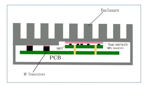
Both the RF functional amplification transistor and the thermal baseplate of BMP module shall contact with the system enclosure closely. The joint shall be filled with qualified thermal gap filler, and the heat shall transmit to exterior of the sealed box in time to make sure the RFPA operates within the normal temperature range.
